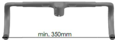
Figure 37 Illustration of the handle area that must comply with the minimum overall width of 350 mm
